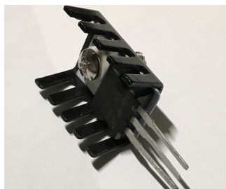
Figure 35. Heatsink on a TO-220 module
